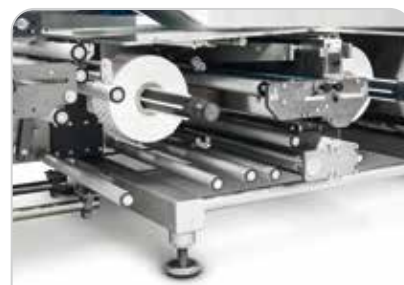
Front-loading reel holder that facilitates loading of the reel
